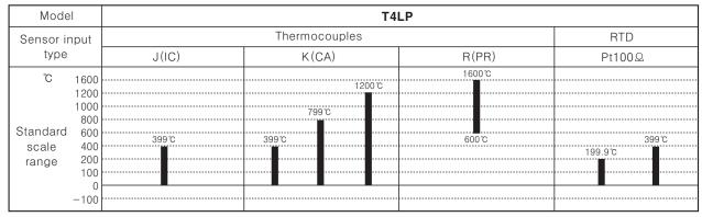
\*In case, the sensor is R(PR) type, it is not available to indicate the temperature and control correctly.
