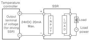
\*When using voltage (for driving SSR) in the other purposes, do not exceed the range of the rated current.
