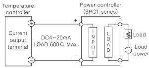
\*The current value of DC4-20mA is available at lower than  $600\Omega$  of resistive load.
